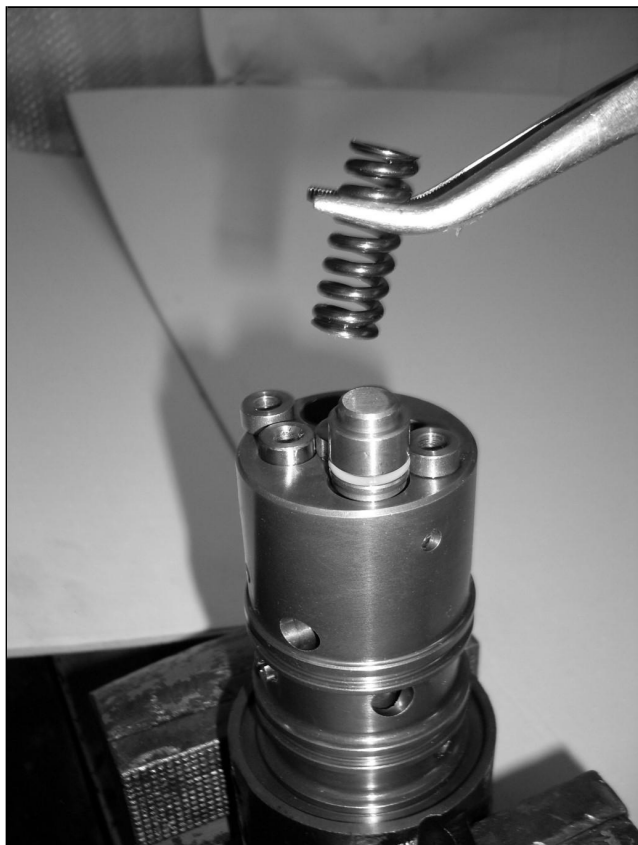
Fig.31 Remove the spring, the ball and the two spacers.
